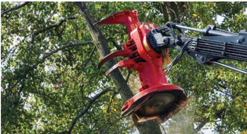
Central Tree pairs a new Quadco 22SC high-speed saw with its TimberPro TL745D feller buncher.
