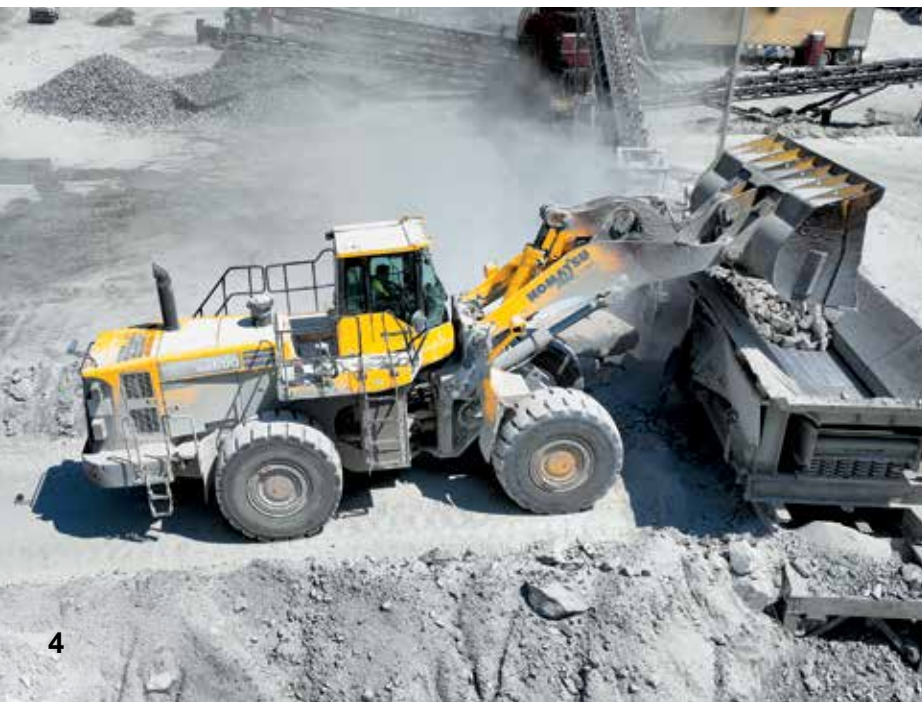
A Shawnee Stone operator feeds a crusher with a Komatsu WA600 wheel loader.
