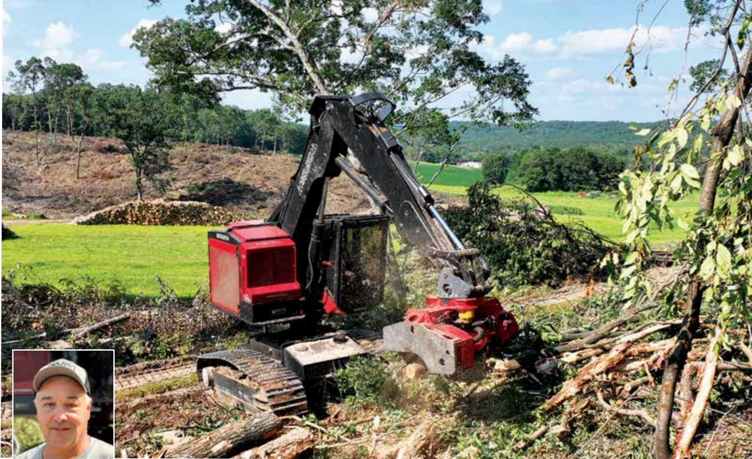
JW Logging operator Craig Stabenow uses a TimberPro TL735D feller buncher with a leveling cab to cut trees to length.
