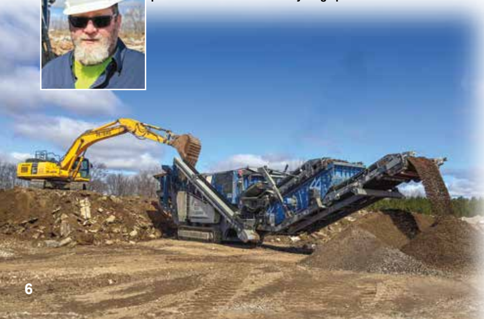
Operator Josh Beyer charges a KLEEMANN MR 130 Zi EVO2 mobile impact crusher with a Komatsu PC360LC excavator as part of Peters Concrete's recycling operations.
