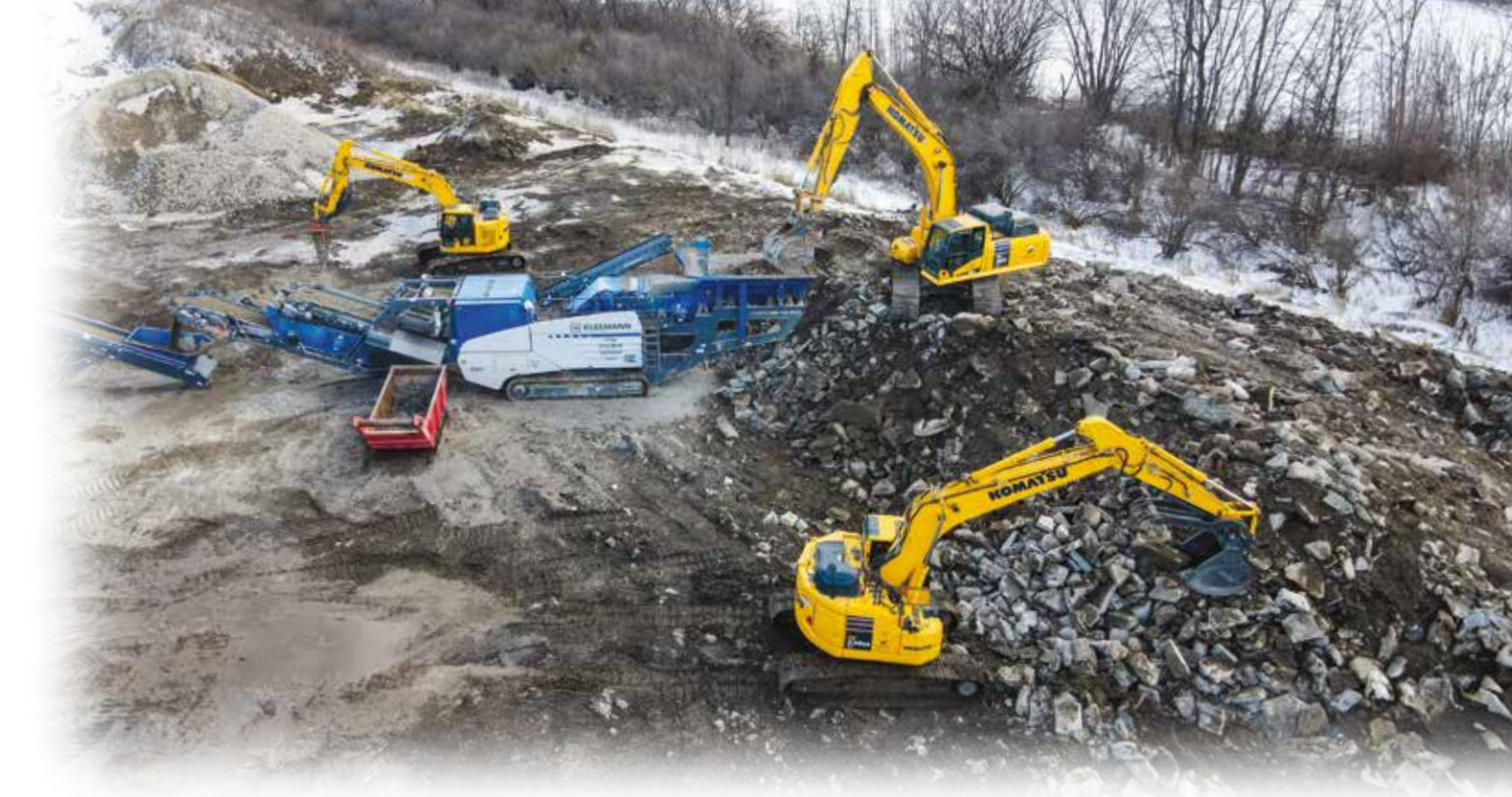
Kinney Contractors recycles old concrete at its yard in Springfield, Ill., using its Komatsu excavators and a KLEEMANN MR 130i EVO2 mobile impact crusher rented from Roland Machinery Company.
