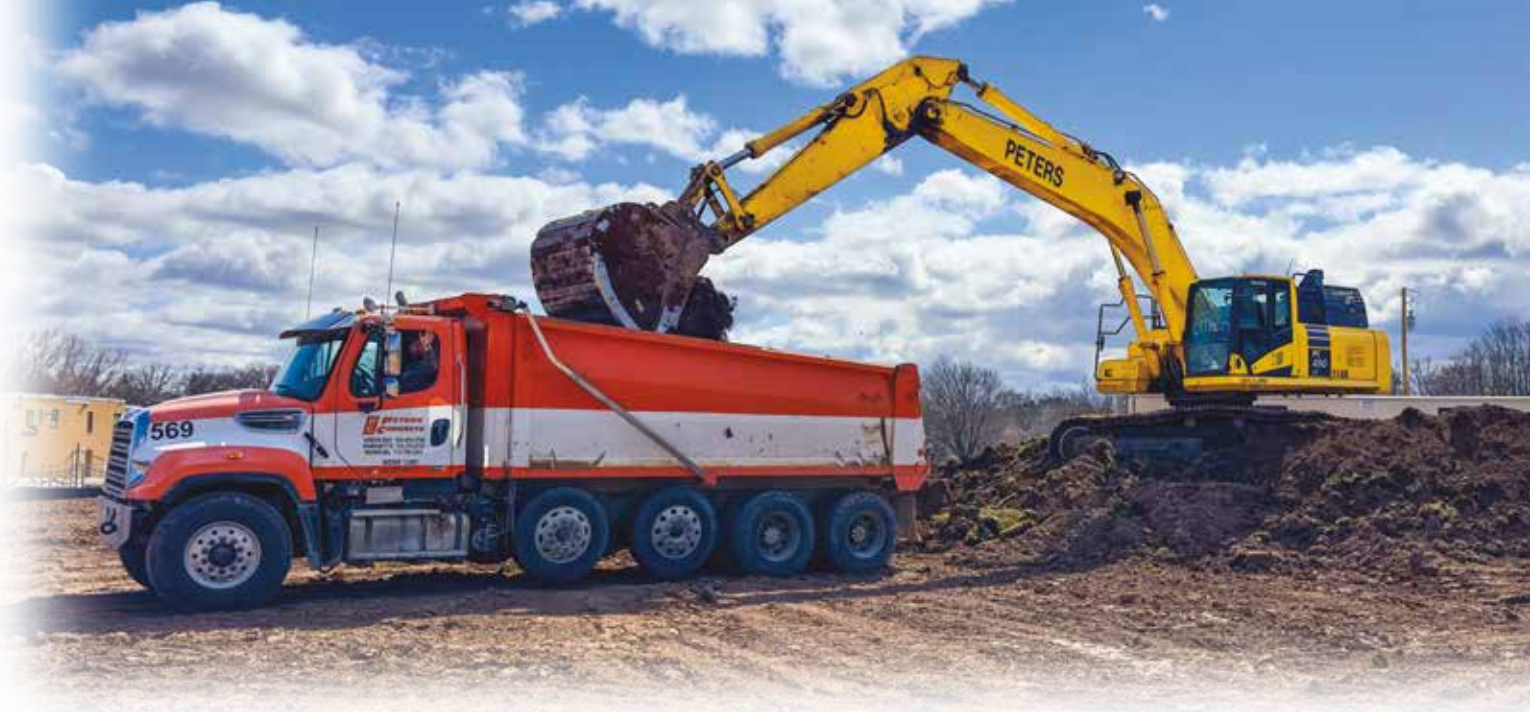
An operator moves dirt and loads trucks with a Komatsu PC490LC excavator.
