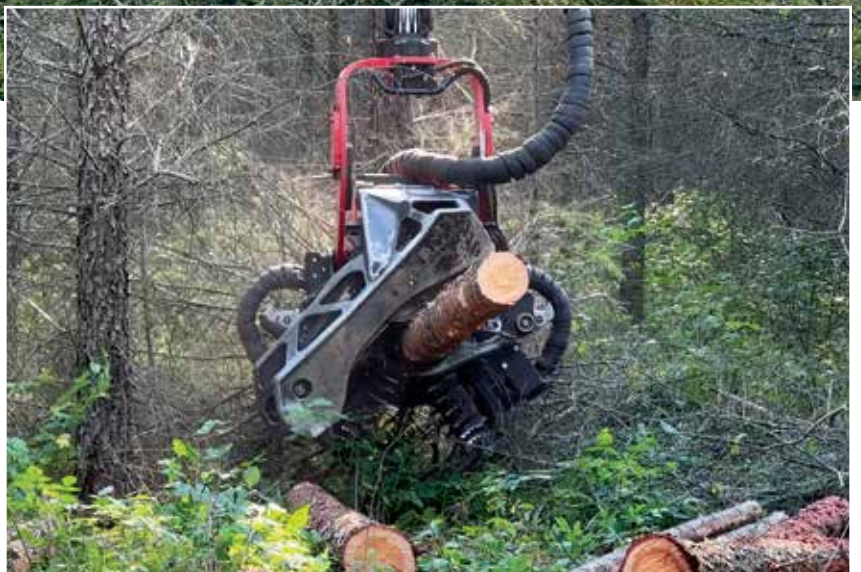
A&A Forest Products owner Anthony Cary cuts larch with a Komatsu 931XC-3 harvester equipped with a Komatsu C144 harvesting head.
