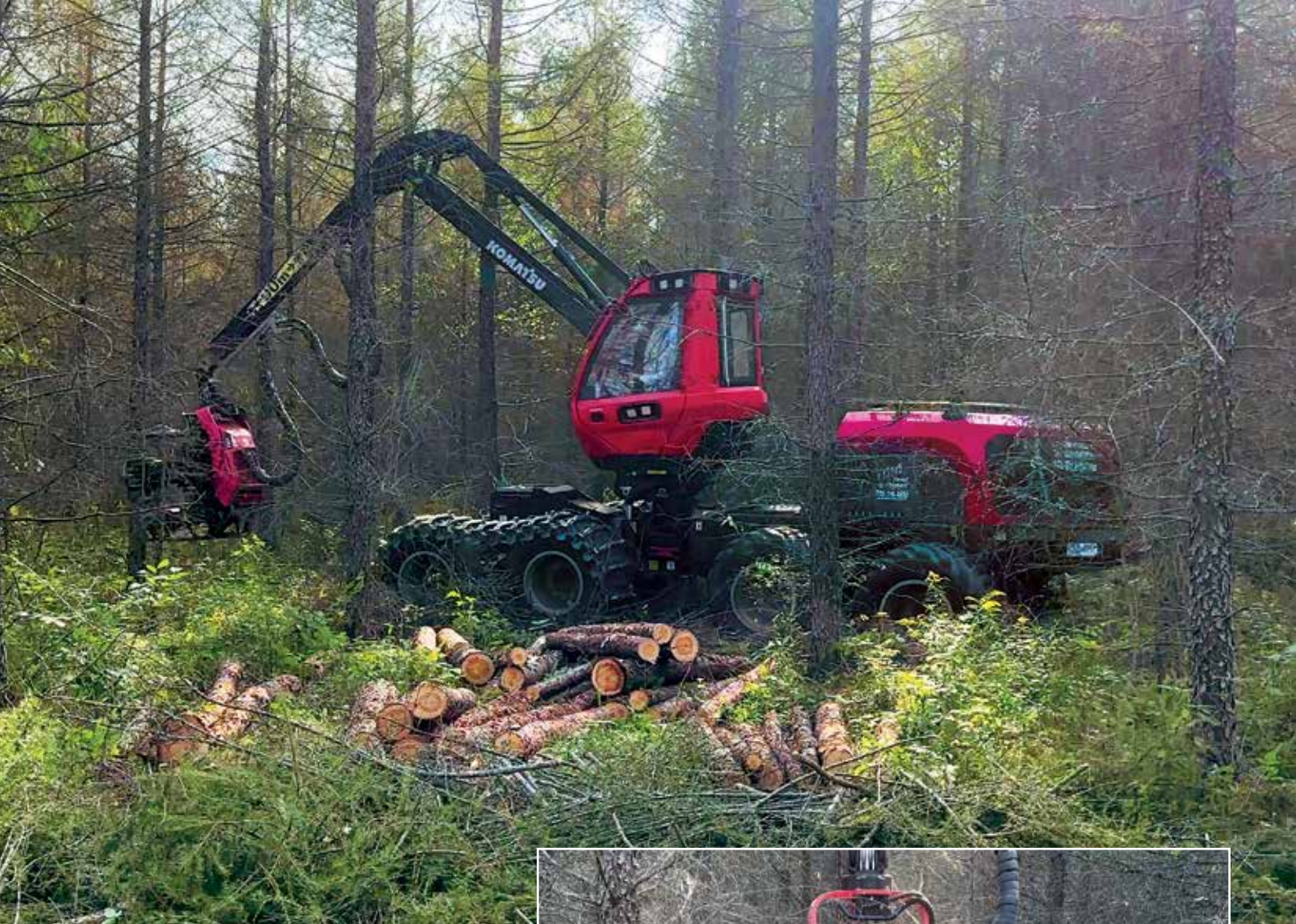
A&A Forest Products owner Anthony Cary cuts larch with a Komatsu 931XC-3 harvester equipped with a Komatsu C144 harvesting head.
